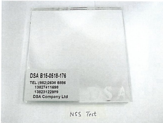
Photos of test specimen before neutral salt spray test.
