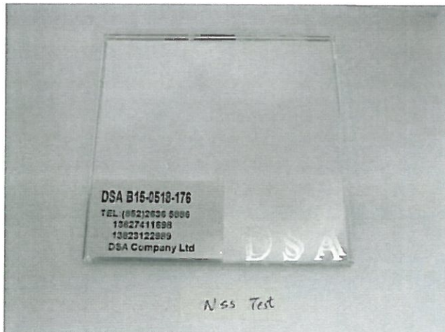
Photos of test specimen after neutral salt spray test for 24 hours.
